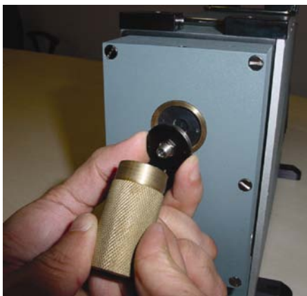
Figure 31: Fitting SMA connector over Slit Disc
