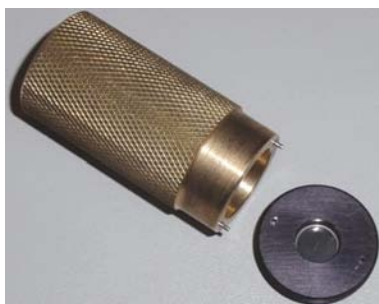
Figure 28: Slit disc & brass insertion tool
