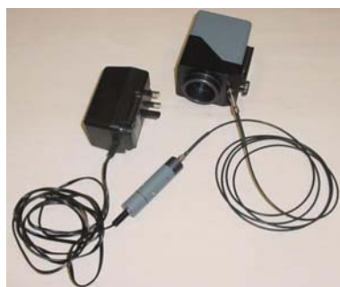
Figure 41: Aiming laser fitted to Collector/Collimator
