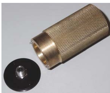
Figure 27: SMA connector & brass insertion tool
