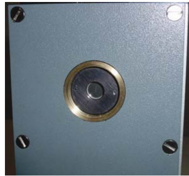
Figure 30: Shutter housing fitted with Slit Disc only
