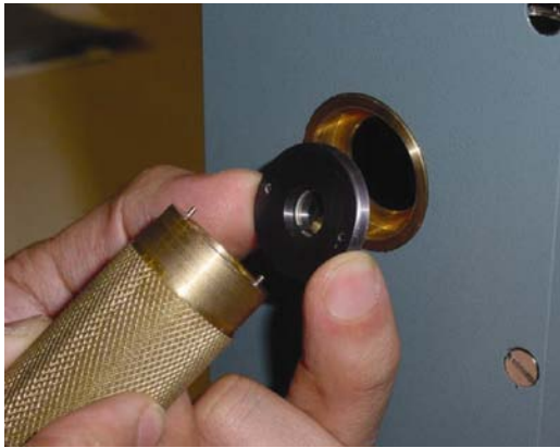
Figure 29: Inserting Slit Disc
